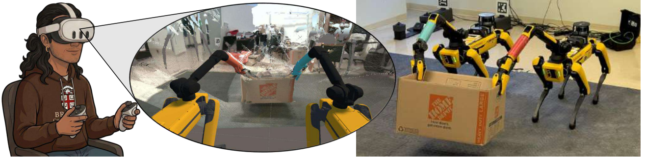
Fig. 1: GHOST enables single-operator dual-robot control. Our VR teleoperation system enables individual or simultaneous dual-robot control to perform complex mobile manipulation tasks, with a 3D virtual scene reconstructed and rendered in real time from onboard cameras.
