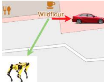
Figure 4.4: An illustration of the ground vector and the figure vector, depicted as the green and the red arrow, respectively, computed by the spatial predicate grounding (SPG) module (Section 4.4.3) to resolve the spatial referring expression “the red car to the right of the bakery.”
