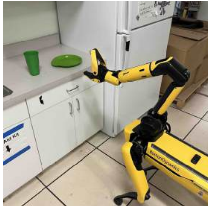
Figure 1.1: An example of robotic language grounding where the robot must associate the word “cup” with the green cylindrical object in front of it, and the word “fetch” with the motion of grasping the “cup” and delivering it to the user to complete the natural language command “Hey robot, can you fetch me the cup?”
