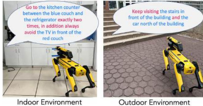
Figure 4.1: Our system Lang2LTL-2 grounds spatiotemporal navigation commands in indoor and outdoor environments. The spatial and temporal components of the example commands are highlighted in blue and red, respectively.
